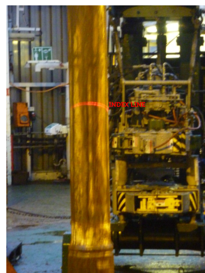
Fig. 3 An index (or zero) line was made on the pipe; the compensated laser was used as a reference point when measuring the "passes" of DEPTH-LOC across the known depth of the pip tag.
