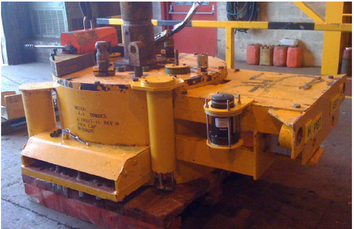
Fig 4. Tree Cap c/w Metrol's Modem and SMM
