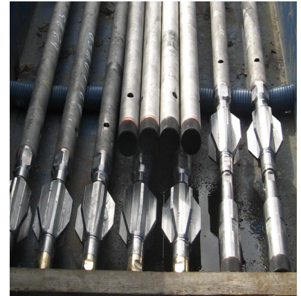
Fig 1. Metrol internal gauge carriers and repeater stations.
